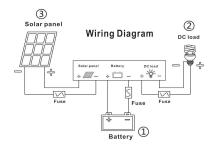
① Connected with Battery first; ② Connected with Load; ③ Connected with Solar Panel.
